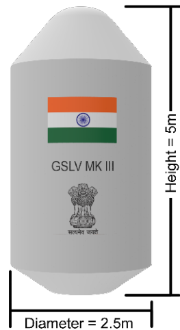
(b) Dimensions of payload fairing
