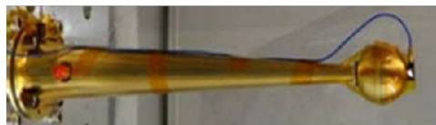
Figure 36: Electric Field Sensor
